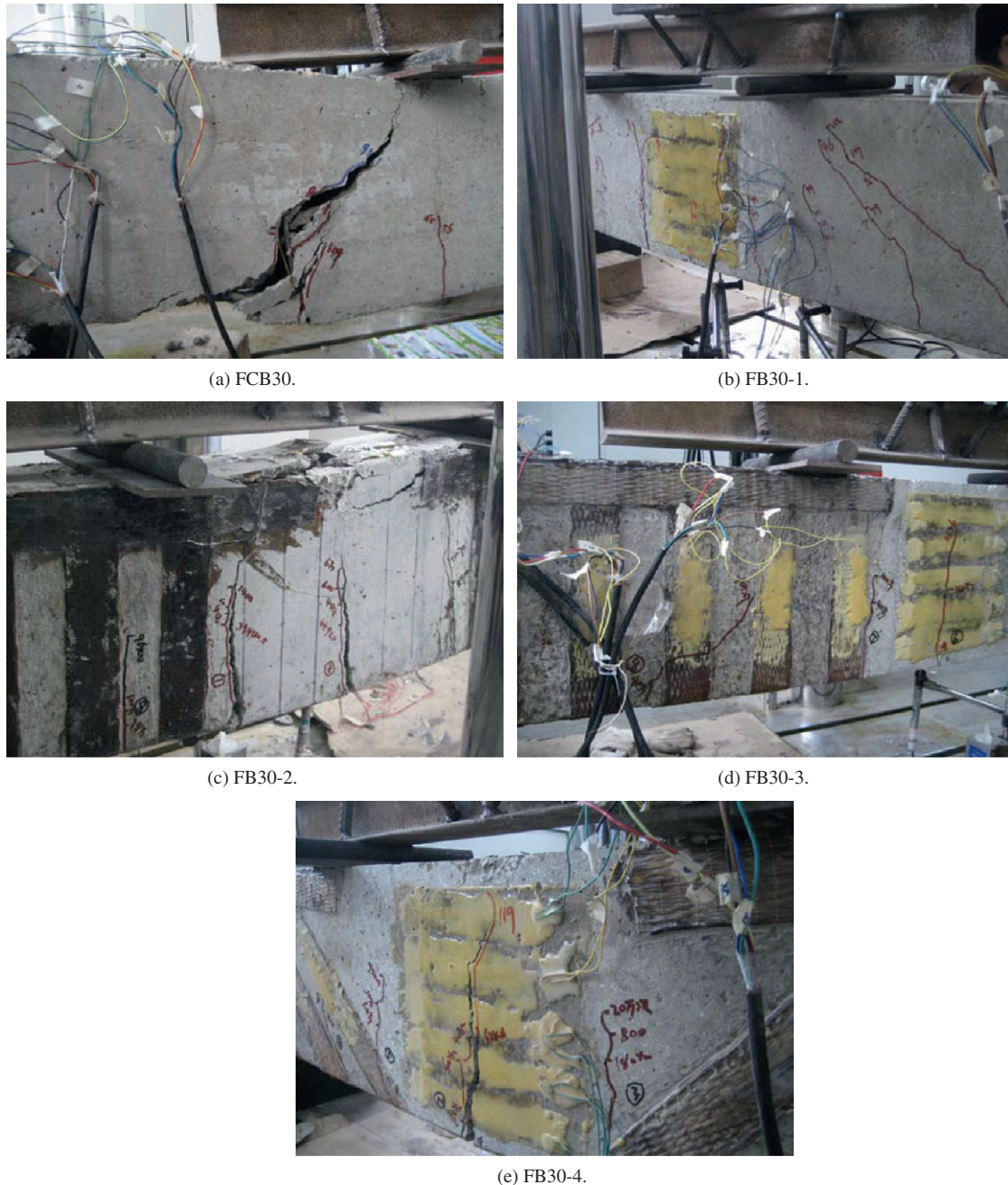
Fig. 5. Failure modes of the beams tested.
